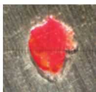
Dirt-in-paint defects under the light-optical microscope
